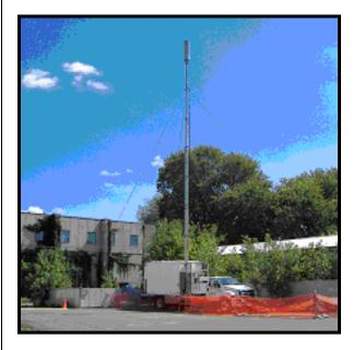
It is best to locate portable towers, such as the one pictured above, away from campgrounds as they require a significant footprint and are powered by generators.
